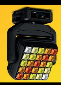
With 900 W of total power, the versatile MagicPanel-FX has 25 next-generation RGBW high-power LED emitters and an active phase-change liquid cooling system using a heat pipe for intensive use in "wash light" mode. The continuous, unlimited, rotation on pan and tilt, first introduced on the legendary MAGICPANEL-602 in 2013, is standard. MAGICPANEL-FX has serial connectivity and can be controlled using DMX-RDM, ArtNet™, sACN or wireless CRMX TiMo RDM by LumenRadio™.
